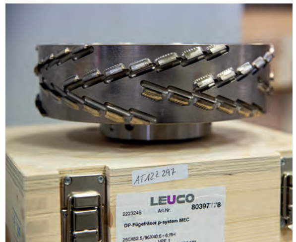
It was now the logical consequence to integrate LEUCO p-System tools with a 70 degree shear angle on the new line.
