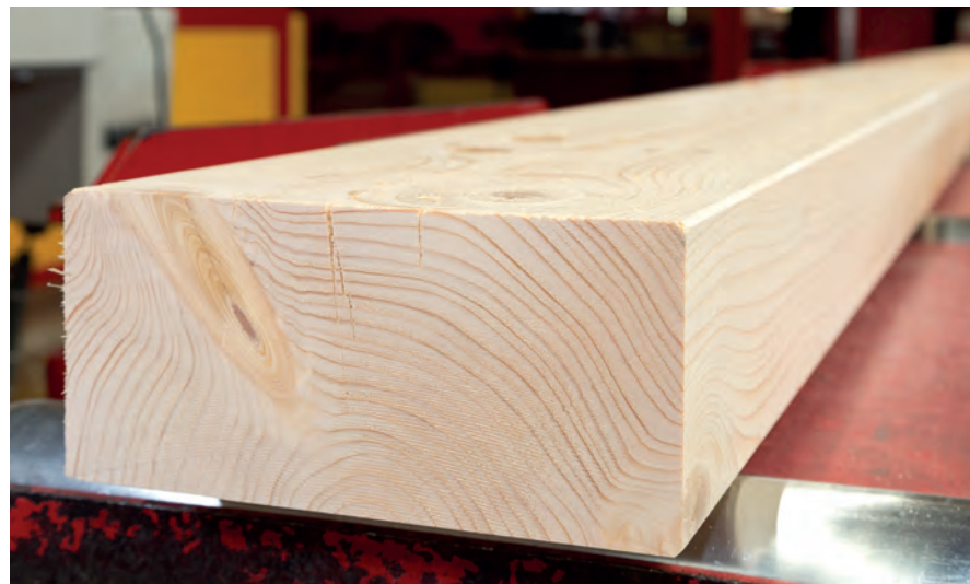
It is not necessary to rework the accurate cuts which can be used as visible edges. With this saw blade, customers can perform operations that previously required a milling cutter. In this way, they save machining time on the joinery center.
